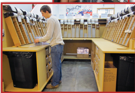
What a contrast! Stacks of batchwork before and now fast and simple one piece flow! Building just what you need when you need it. One piece flow is counterintuitive. Batchwork seems faster and more efficient but it is just the opposite. In this picture we show one of our many U-shaped Lean cells throughout our facility.
