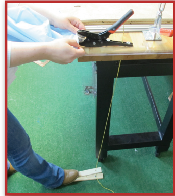
Using your head, not your wallet. This simple improvement uses a string attached to a home-made wood pedal, and a pair of pliers as a crimping tool. The operator's hands are now free and so is his mind to think of the next great improvement.
